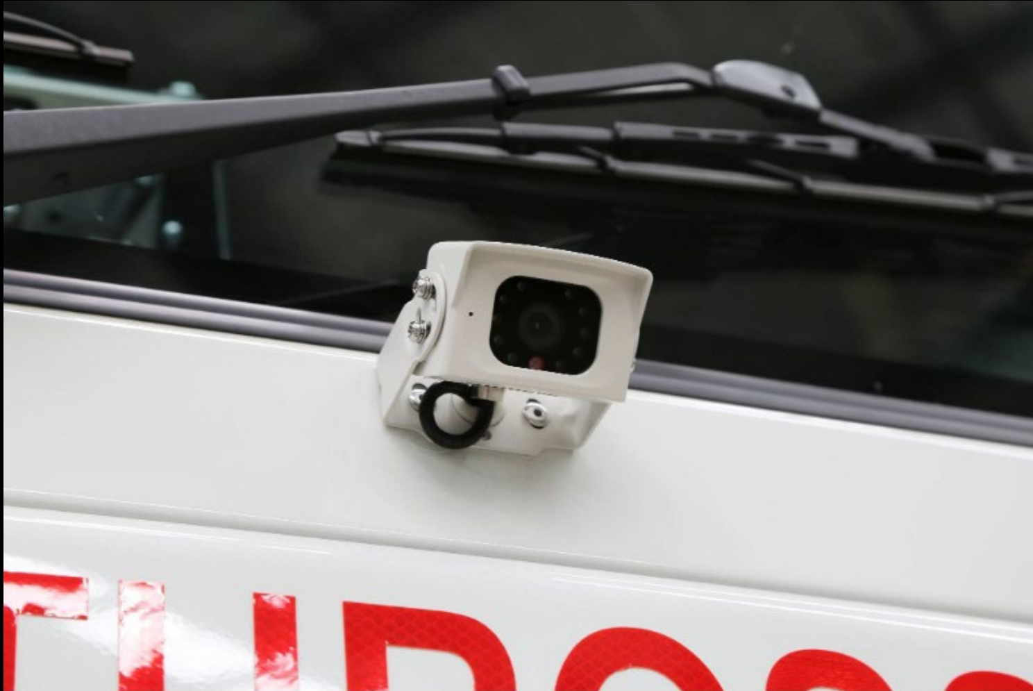
Front facing camera – viewable from vehicle media display along with rear/reversing camera.
